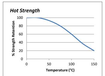
"Hot strength" shear strength tests performed on mild steel. Fully cured specimens conditioned to pull temperature for 30 minutes before testing at temperature. ET5429 can withstand higher temperatures for brief periods (such as for paint baking and wave soldering processes) providing the joint is not unduly stressed. The minimum temperature the cured adhesive can be exposed to is -40°C (-40°F) depending on the materials being bonded.
