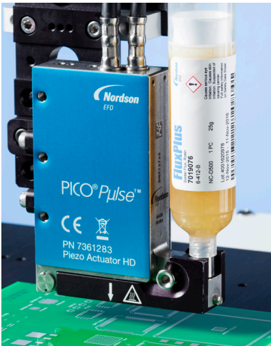
PICO Pulse® jetting FluxPlus onto a PCB.
