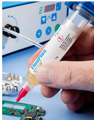
Performus™ X100 dispensing FluxPlus onto a PCB.
