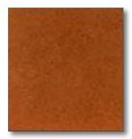
Prior to the advent of J-STD-004B, the prevalent test for halides/halogens in flux was through the use of silver chromate test paper. A drop of flux is deposited on the paper, and if the paper does not turn white or yellow, it is a confirmation that no halides are present. **WF-9942** PASSES the silver chromate paper test for halides.
